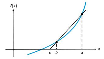
If c isn't a root, but f(c) is closer to zero than f(b), then b is relabeled as a, c is relabeled as b, and the prediction process is repeated. Provided the graph of f(x) is smooth and provided the initial values of a and b are close to a simple root, the secant method rapidly converges to a root.
