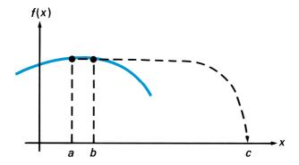
If <u>SOLVE</u> has already found values a and b such that f(a) and f(b) have opposite signs, it modifies the secant method to ensure that c always lies within the interval containing the sign change. This guarantees that the search interval decreases with each iteration, eventually finding a root.
