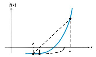
If SOLVE hasn't found a sign change and a sample value c doesn't yield a function value with diminished magnitude, then SOLVE fits a parabola through the function values at a, b, and c. SOLVE finds the value d at which the parabola has its maximum or minimum, relabels d as a, and then continues the search using the secant method.
