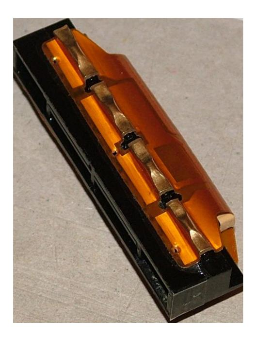
Now you're done with the hard part of the job, just replace the refurbished I/O block and reassemble your HP-41.
