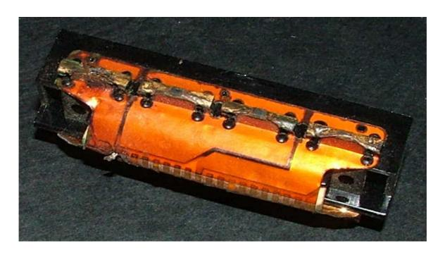
Now remove the plastic rivets that hold the damaged Flex-PCB. A sharp X-acto knife will help a lot here.
