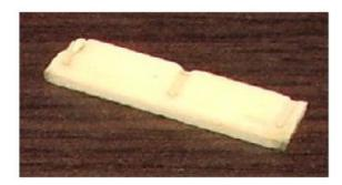
NOTE: I've found some cases in which the sponge has also been damaged to the point to be useless and no longer provides the required pressure to the contacts underneath.
