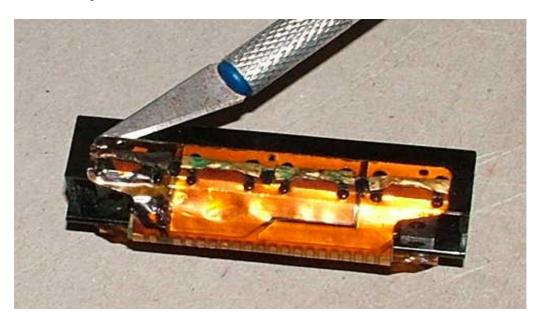
You don't need to cut all the rivets for now, just enough to pull the old PCB off the plastic block.
