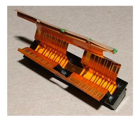
Now tight bend the connectors area of the Flex-PCB around their plastic flanges and apply good presure again to ensure proper adherence. First the outer ones.
