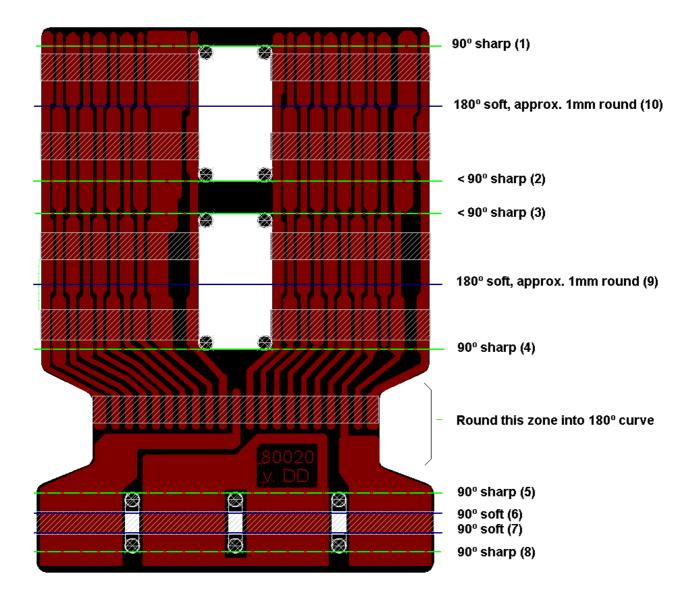
Please pay attention as the accuracy of the refurbishment process relies on the precision of the Flex-PCB folding. It must reproduce the original circuit folding as exactly as you can.
