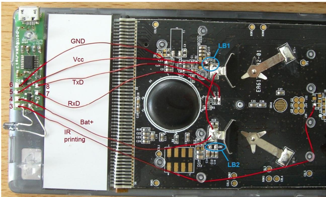
First, however, two components must be removed from the main board:
