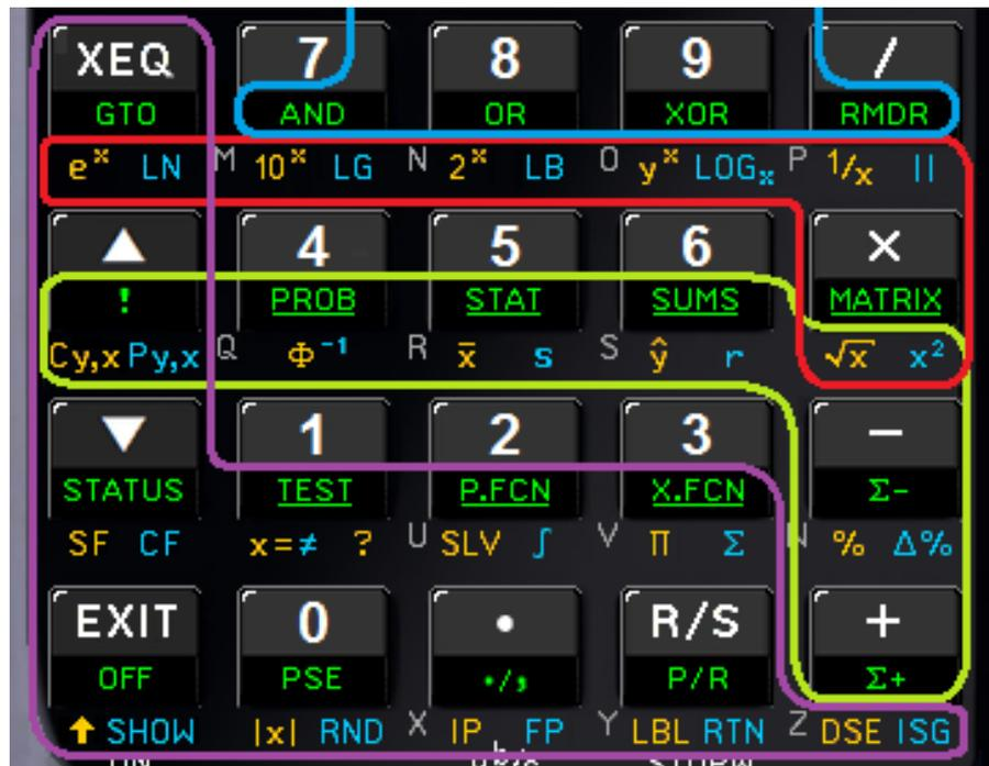
products and sums, keys for EXITing programming mode and for pausing program execution (PSE), some commands for extracting parts ( $|x|$ , IP, and FP), keys for
