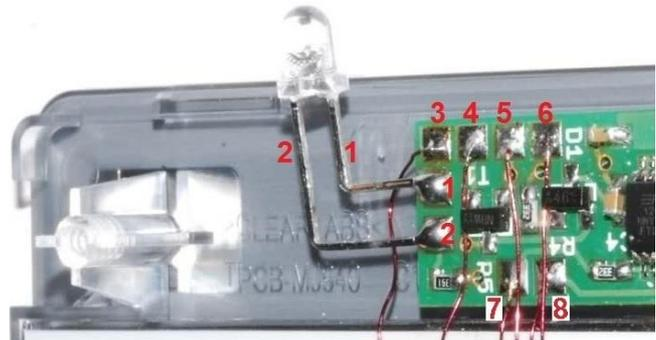
Solder the formerly longer diode leg to terminal 1. Solder the other one to terminal 2.
