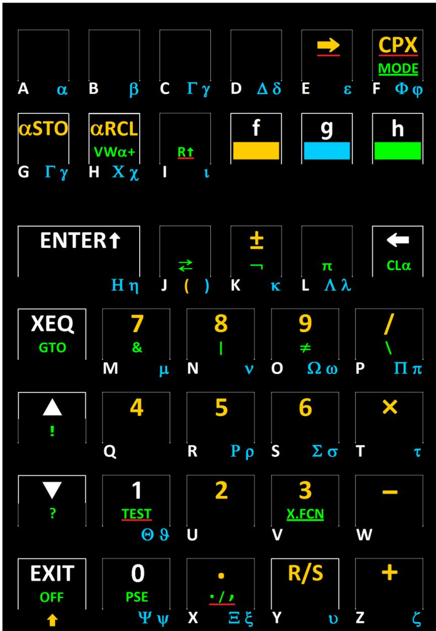
The labels underlined in red call alpha catalogs. Labels underlined in green and labels shown between heavier white key contours do not append characters to *alpha* directly – all other labels do.
