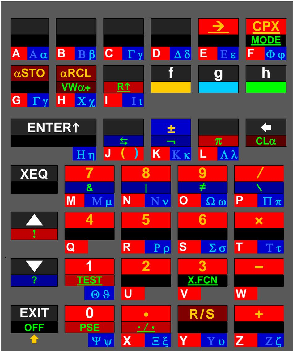
The alpha catalogs called by **f**  $\rightarrow$ , **f** **CPX**, **R**  $\uparrow$ , **.**/**.**, and **TEST** feature even more characters (see p. 132). Check the [IOP](#) for  $\alpha$ STO,  $\alpha$ RCL, VW $\alpha$ +, and more alpha commands.
