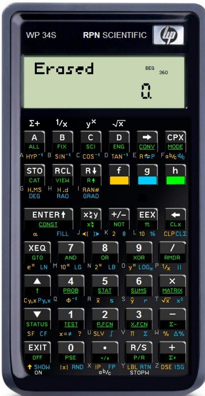
Look at [the keyboard of an HP-42S](#) for comparison. The most striking difference to it is the colorful surface of your *WP 34S*. You get five functions per key on average. White print on key top is for the *primary* function of the key. For *secondary* functions, green labels are put on the slanted lower faces of 34 keys, golden and blue labels are printed below them on the *key plate*. Grey letters are bottom left of 26 keys.
