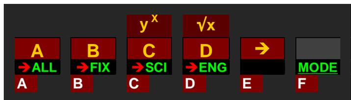
Calculating in bases 11 ... 15, those keys not needed for numeric input will work as shown in the first picture above. In any integer base, attempts to enter an illegal digit from the keyboard – such as e.g. 4 in binary – will be blocked.
