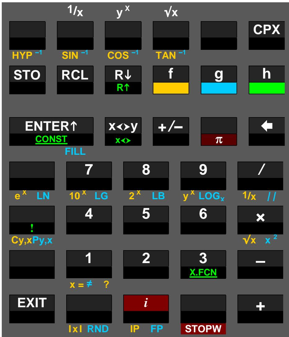
After pressing **CPX**, your WP 34S allows for the complex operations shown on this *virtual keyboard* (but STOPW represents an application in real domain, see p. [145](#)).
