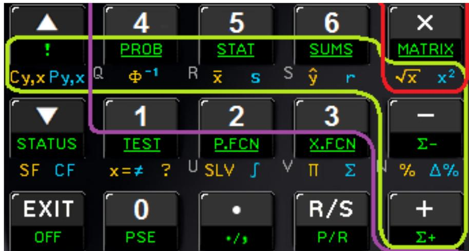
The shifted functions of  $\boxed{4}$  cover statistical distributions: standard normal  $\boxed{\Phi}$  and its inverse  $\boxed{\Phi^{-1}}$ , as well as the catalog  $\boxed{PROB}$  covering nine more continuous distributions and three discrete ones. All these functions have a few features in common:
