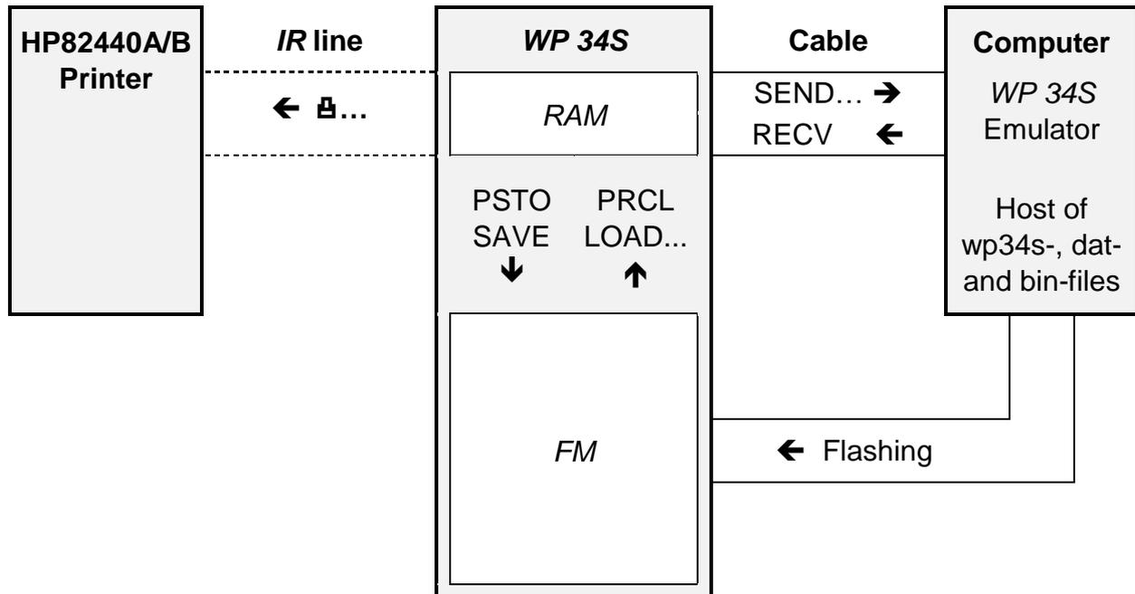
SAVE is for battery-fail-safe internal backup of your work as explained on p. [72](#). The different flavors of LOAD are for recovering from backup. Alternatively to the commands SAVE and LOAD, you may hold down **ON** (i.e. **EXIT**) and press one of the following keys twice:
