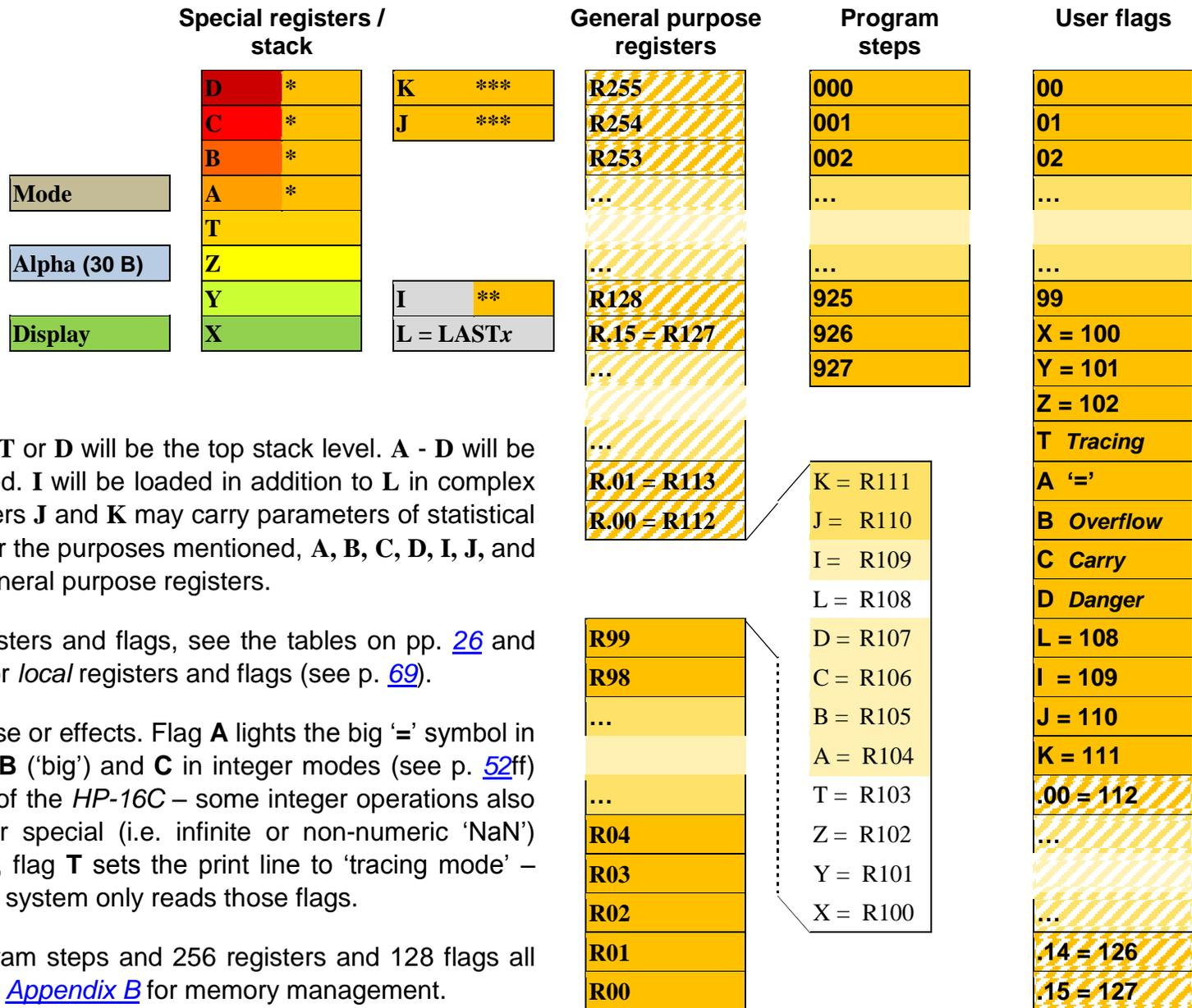
Offering two stack sizes, either **T** or **D** will be the top stack level. **A - D** will be allocated for the stack if required. **I** will be loaded in addition to **L** in complex calculations (see p. [29](#)). Registers **J** and **K** may carry parameters of statistical distributions. Unless required for the purposes mentioned, **A, B, C, D, I, J,** and **K** are available as additional general purpose registers.
