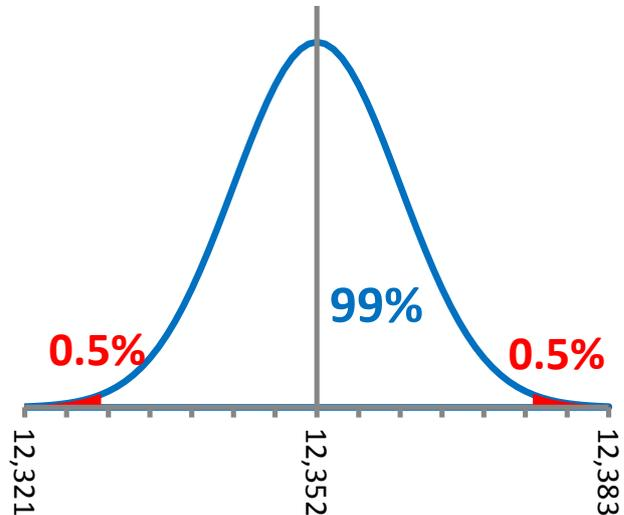
So based on the ten pin sample analyzed, you may expect 0.5% of all pins with diameters smaller than
