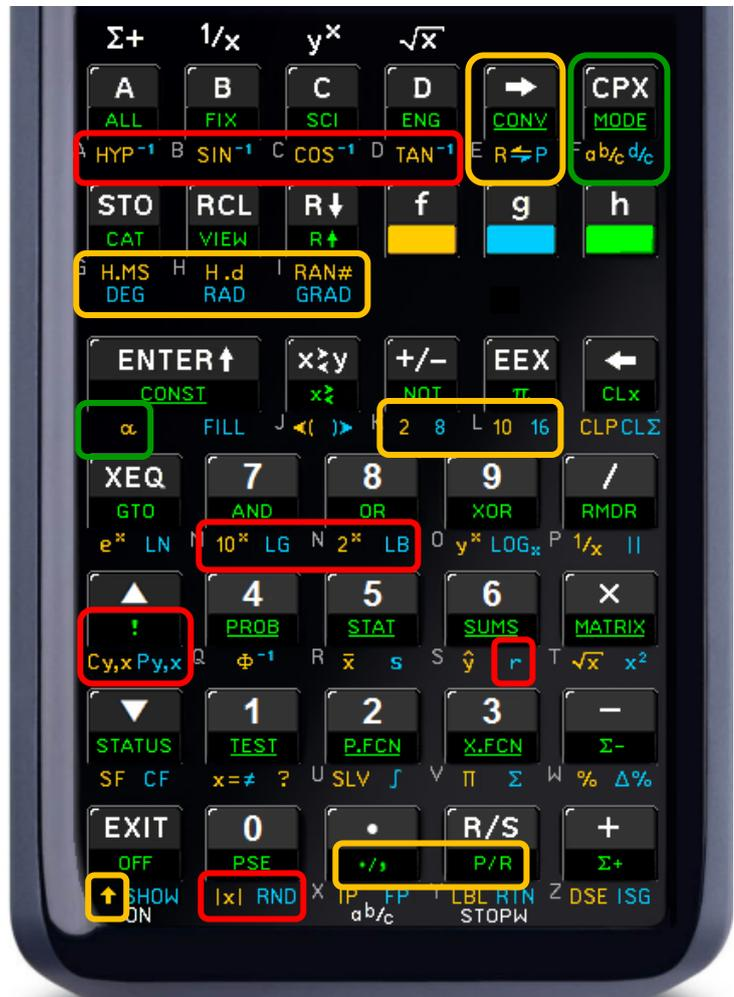
4. **CPX** is for calling complex operations (see p. 29). **a b/c** and **d/c** enter fraction mode for proper or improper fractions (see PROFRC and IMPFRC).
