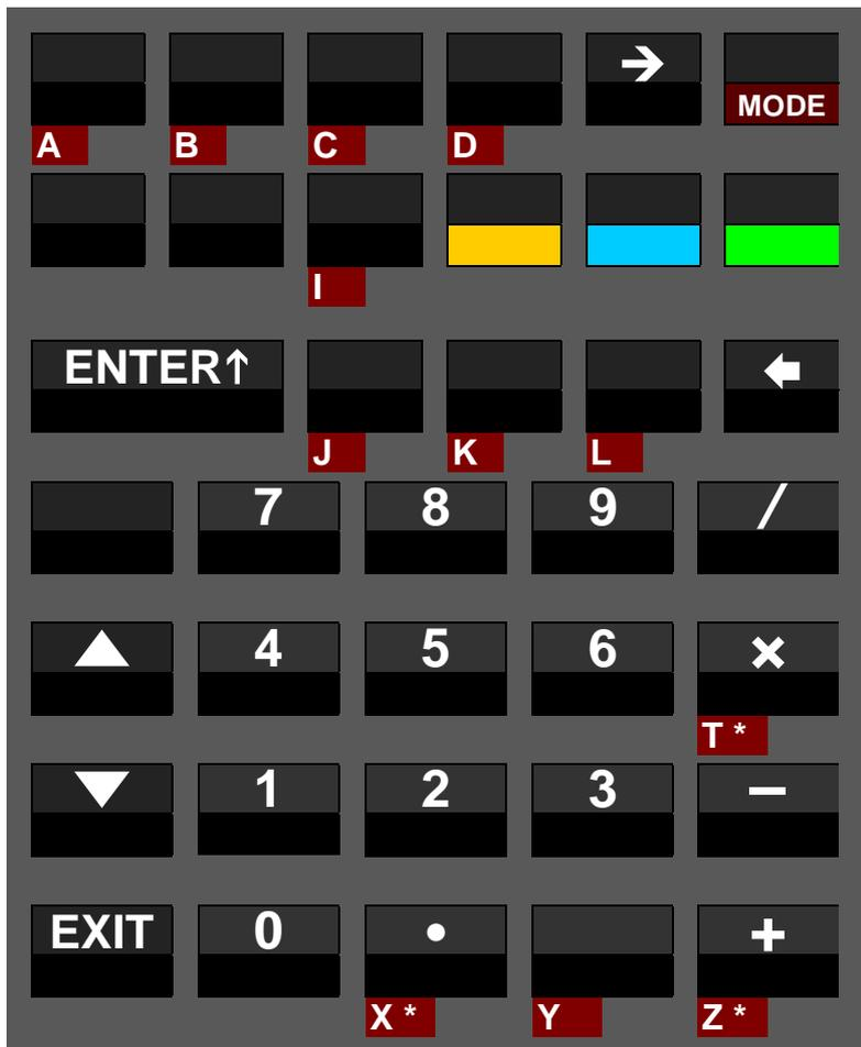
This kind of picture is called a *virtual keyboard* since it deviates from the physical (or real) one of your WP 34S. In such a picture, **dark red** background is used to highlight changed key functionality. White print denotes primary functions also on virtual keyboards, such as the top left key entering the letter A in  $\alpha_T$  mode directly. On the other hand, what is printed white on your physical WP 34S is called a default primary function.
