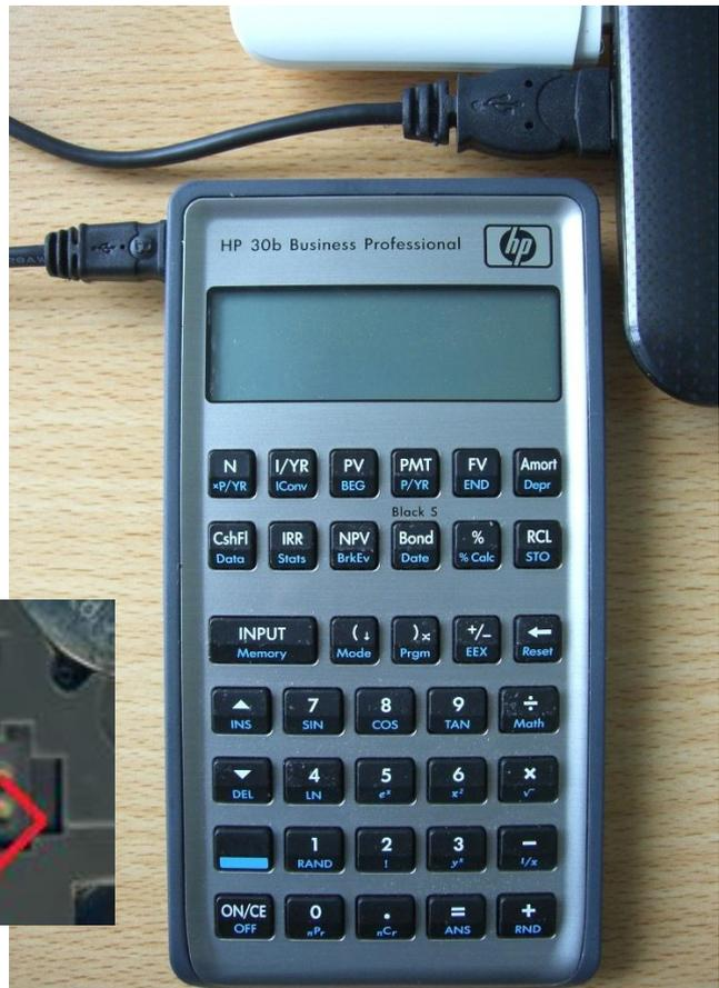
B7. Remove the shorting link. Press RESET to turn your calculator off again.
