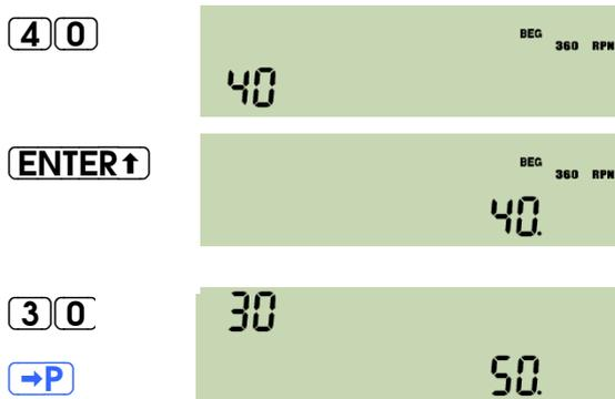
This key separates the two numbers in input here.<sup>7</sup>
